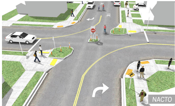
Diverters can be used to manage volume on Bicycle Boulevards
