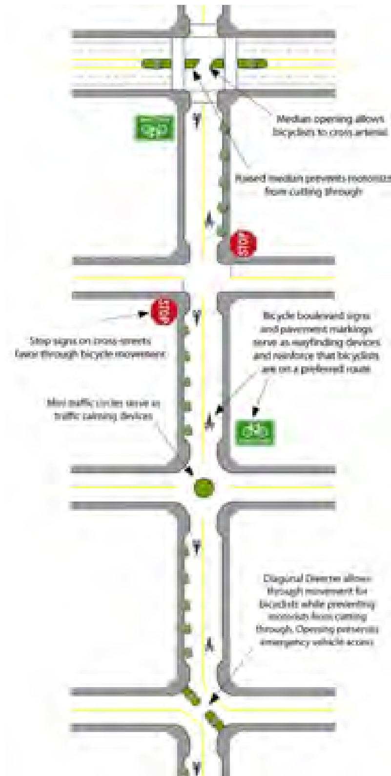
Figure 6.8 – Example Elements of a Bicycle Boulevard
