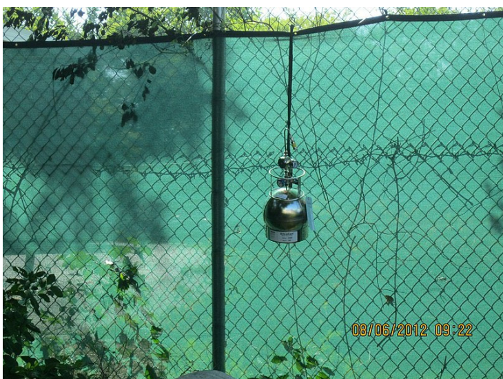
Figure: example of an air sampling canister deployed at a park
